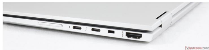
Right: Volume rocker, 2x USB Type-C + Thunderbolt 3, DriveLock, HDMI 1.4
