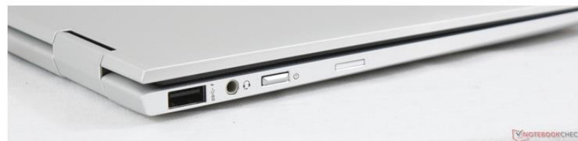
Left: USB 3.1 Type-A, 3.5 mm combo audio, Power button, Nano-SIM slot (optional)
