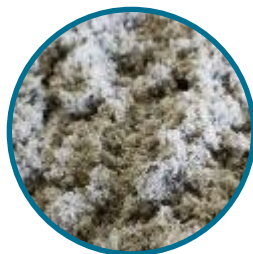
Cellulose \lambda \approx 0,038 \text{ W/mK}
