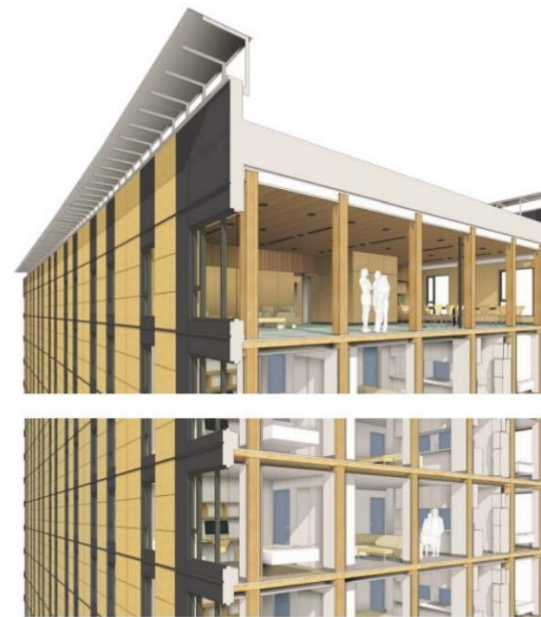
exposed mass wood structure
