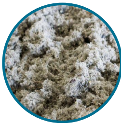
Cellulose \lambda \approx 0,038 \text{ W/mK}
