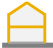
Ossature bois (murs/charpente/planchers)
