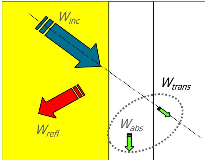
$$R(\text{dB}) = 10 \lg \frac{W_{\text{incidente}}}{W_{\text{transmise}}}$$
